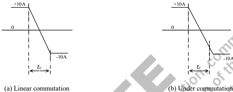
Fig. 1.21: Coil current versus time during commutation
